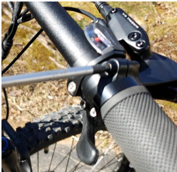
Levers, shifter, and display positioned on the bar
