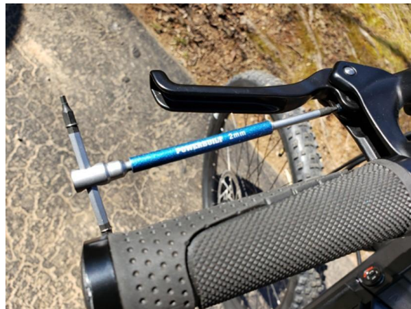
Setting brake-lever reach
