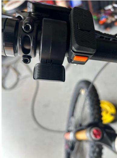
Thumb throttle (if equipped), just inboard of the left grip
