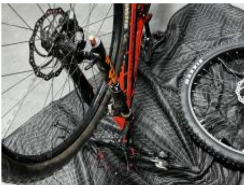
Guiding the rotor into the caliper
