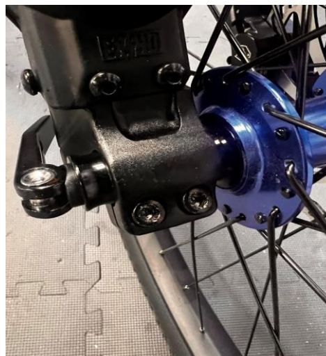
Front thru-axle and hub
